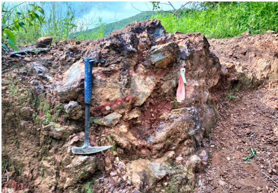
Figure 22. Veta Norte Sur. Mineralized breccia in historical working. Sample site 24588, which returned 2.21 g/t Au over a 1.5m width (photo courtesy of Pacific Mining Services).
