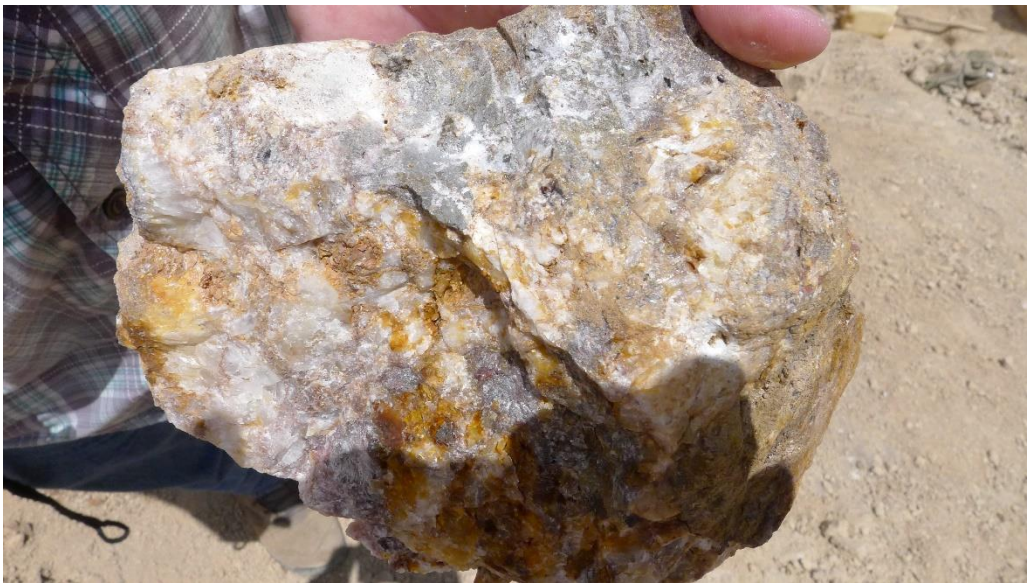
Figure 11. Quartz vein from floor of gambesino workings, La Dolorosa. Sample contains free gold, as does the pulverulent, hematite-rich material in the adjacent structure (Bow, 2021).
