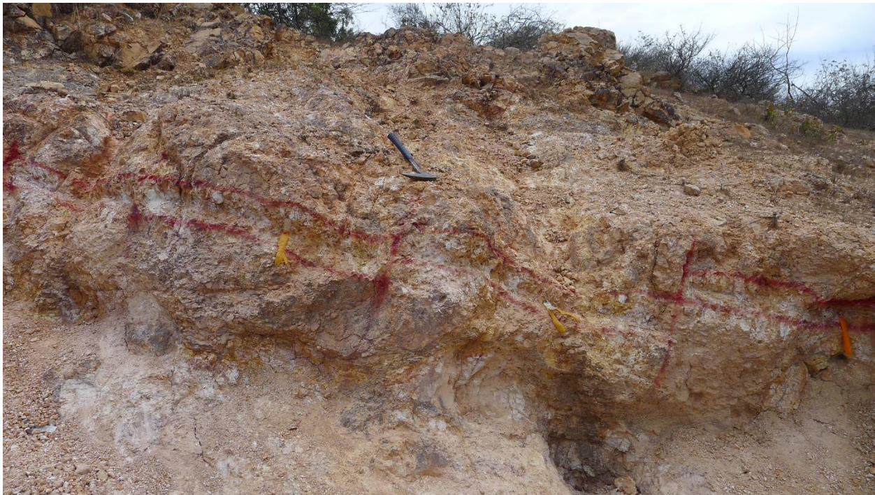
Figure 25. Sub horizontal chip channel line, illustrating the use of paint, flagging, and metal tags as controls to sample locations.
