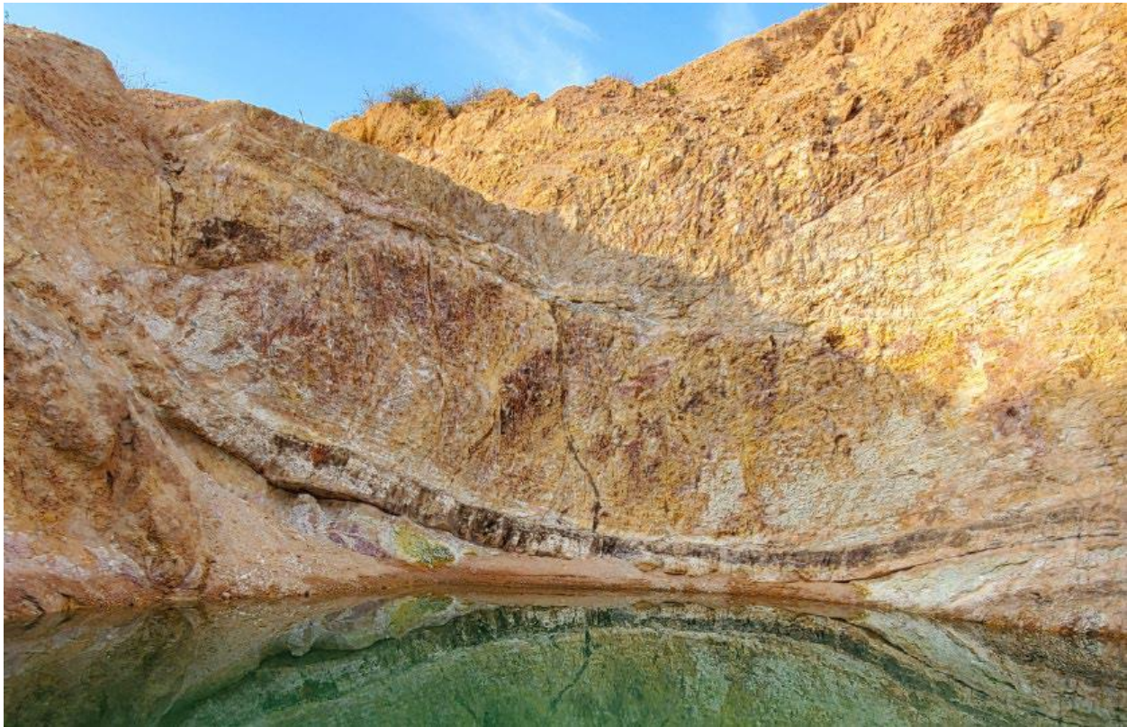
Figure 17. North wall of the El Polo pit, illustrating the low angle breccia which has been the target of recent gambesino mining efforts. Note intense alteration and moderate to high angle fracturing of the hanging wall (Smith, 2020).
