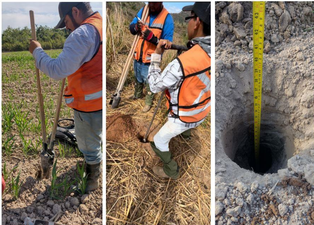
Figure 26. Sampler breaks ground with a post hole digger prior to initiation of auger drilling.
